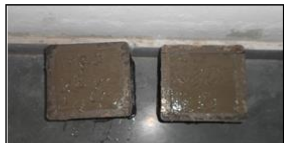
Figure 8: Concrete Cubes Casting
