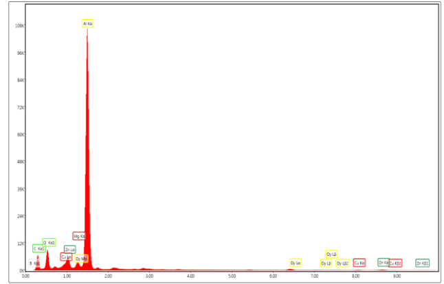
Fig. 5 EDS profile analysis for the composite with 0.5% B 4 C and 0.5% of Al 2 O 3 nano reinforcements.
