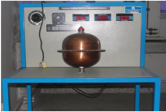
Figure 3: Insulating powder apparatus
