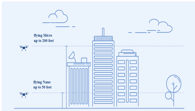
Figure 1. Flying range of nano and micro drones (Directorate General of Civil Aviation, Government of India, 2021)
