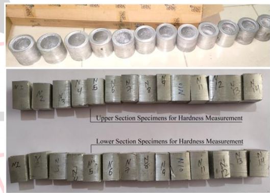
Fig 7: Casted Cylinders and Hardness specimen cut from the cylinders
