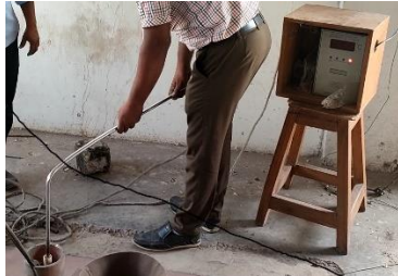
Fig 3: Temperature measurement of Metal (Converted in to liquid phase)
