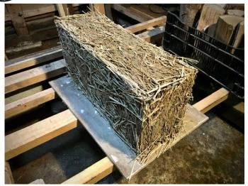
Straw clay blocks, also known as straw bales, are building materials made by compacting straw (typically wheat, rice, or barley straw) with a clay-based binder. The resulting blocks are used as load-bearing or non-load-bearing elements in construction, offering numerous benefits in terms of sustainability, energy efficiency, and environmental impact.
