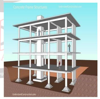
Concrete framed structures are widely used in construction due to their strength, durability, and versatility. These structures consist of reinforced concrete members, such as columns, beams, and slabs, which work together to provide support and stability. Let's delve into some key aspects of concrete framed structures:
