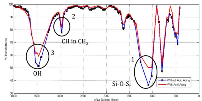
Fig 8 FTIR Spectrum of Samples Without and With Acid Aging
