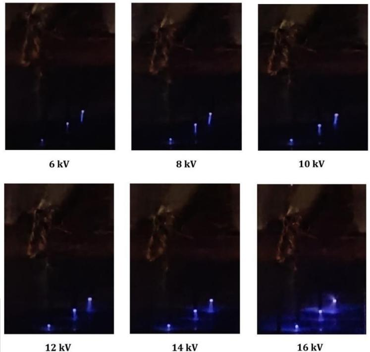
Fig 2 Corona Discharge on the Surface of the Insulator with Different Voltage Levels
