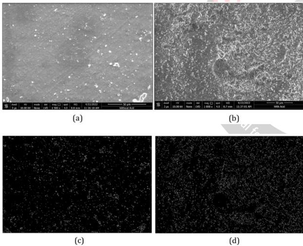
Fig 9 SEM Images (50µm) (a) without Acid Aging; (b) with Acid Aging; (c) Edge Detection without Acid Aging; (d) Edge Detection with Acid Aging
