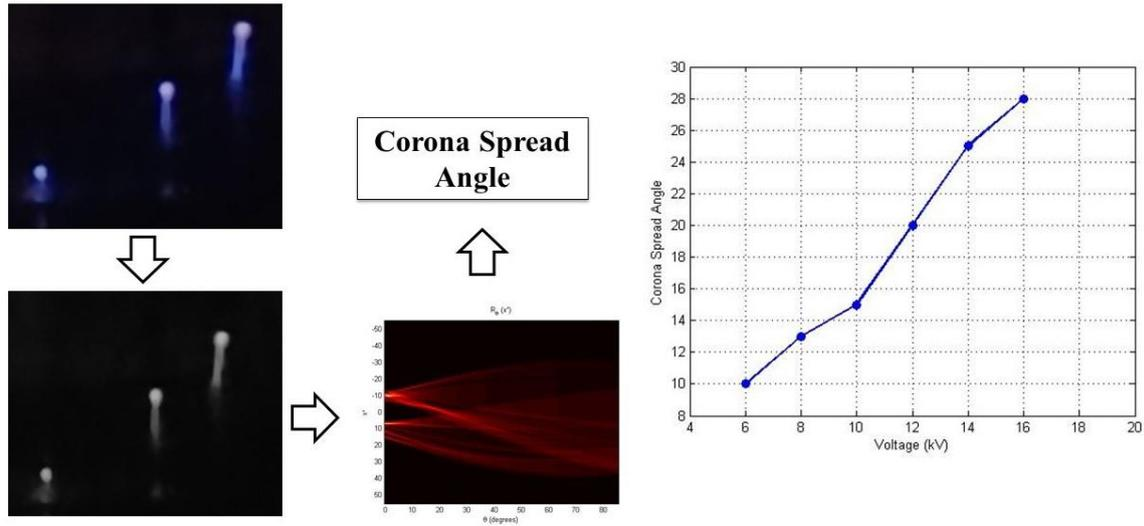
Figure 4 (a) Detection of Hough Lines; (b) Streamer Spread Angle
