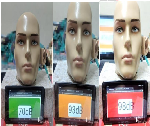
Figure 2: Prototype device with different sound intensity level and colour indication.
