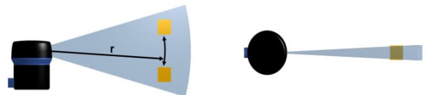
Figure II.6: Vertical arrival angle and slant range
