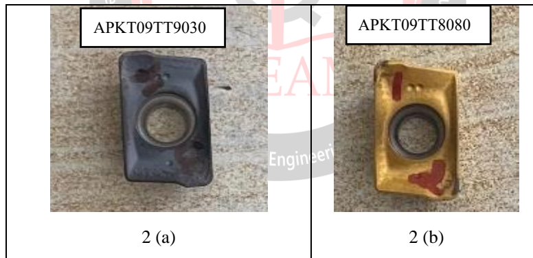
Fig. 2 (a, b) shows TiAlN and TiAlN-TiN coated Tungsten Carbide Inserts
