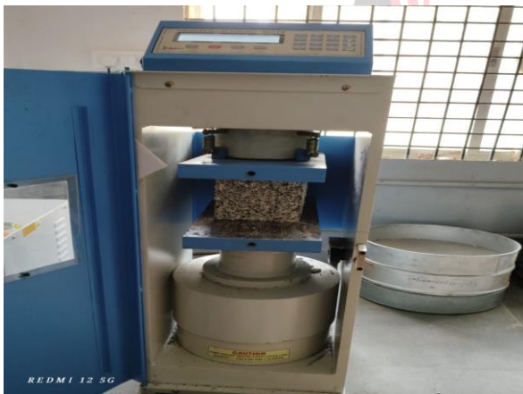
Fig.2 Compression test on concrete cube
