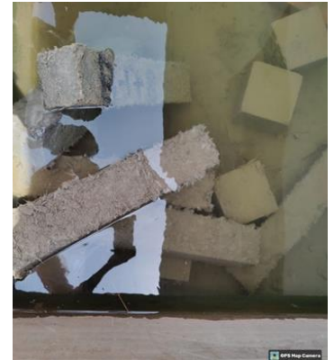
Figure 6. Curing of beam
