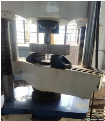
Figure 7. Single point load testing machine
