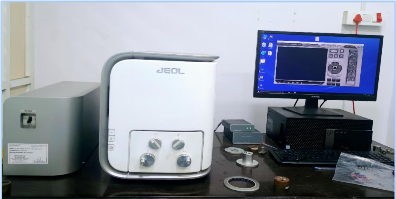
Figure 7: EDS/SEM Analysis machine JEOL 6000 PLUS
