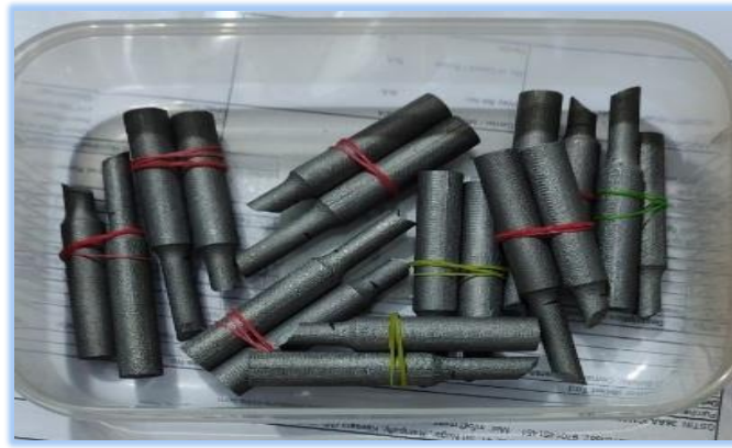
Fig 5: UTM L9 samples after experimental braked samples.
