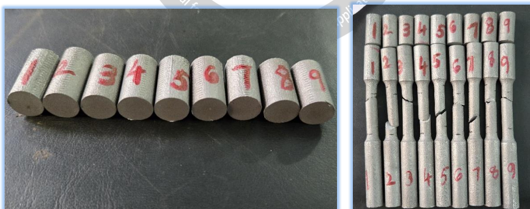
Figure 6: UTM L9 samples and after experimental braked/wire cut samples.
