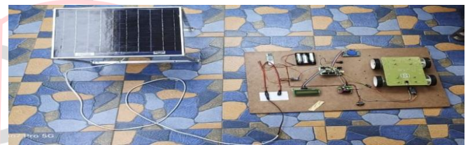
Figure 2: working prototype model of solar base wireless charging station
