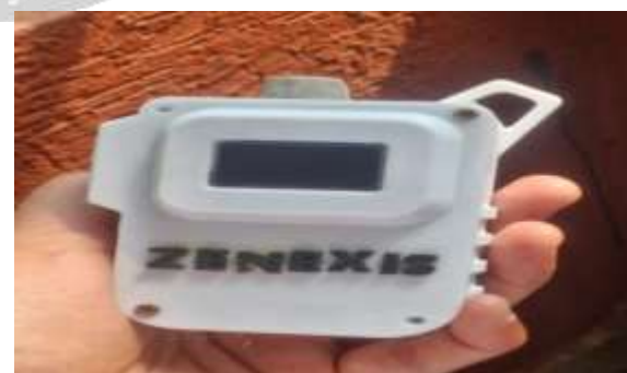
Fig. 3. IoT Device in Weather-Resistant Enclosure for Outdoor Deployment.
