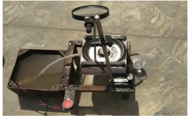
Fig. 9 Working Model of Sea-Water Desalination
