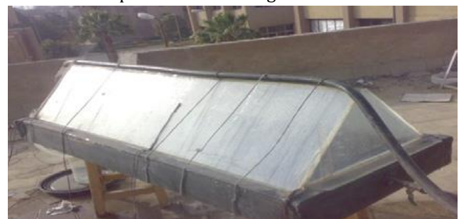
Fig. 7 Passive double slope solar still
