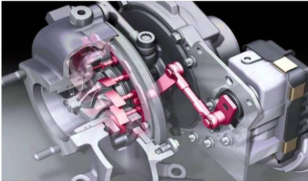
Fig 1: Schematic diagram of Variable Geometry Turbocharger
