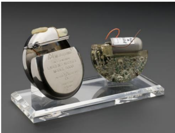
Fig.11 Image of an implantable pacemaker with a radioisotope TEG as the power source [6].
