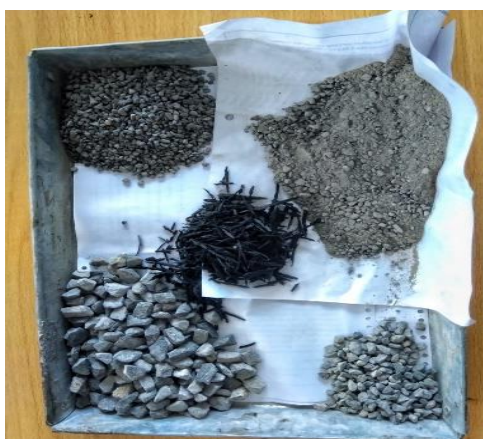
Fig 2. Aggregates, Filler material and crumb rubber
