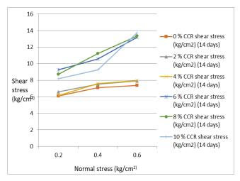
It can be clearly observed that with increase in percentage of CCR added to soil there is considerable increase in the shear strength of soil, with 10% CCR giving maximum shear strength of 11.2 kg/sq.cm.
