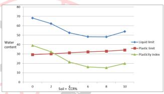
According to past research papers published, the optimum percentage of CCR to be added is 6% to 8%. To obtain the optimum percentage of CCR to be added a graph of percentage of CCR vs. plasticity index is drawn. From the graph the optimum amount of CCR to be added is 7%.
