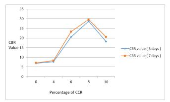
It can be clearly observed that with increase in percentage of CCR added and increase in the curing period of soil, the CBR value of soil has increased significantly. CBR value of soil with CCR is 2-3 times more than the CBR value of soil without CCR.
