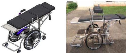
Fig. 2. The isometric view of the designed and developed wheelchair on cad Software (left) and prototype of device (right) [3]
