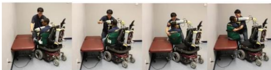
Fig. 14. A sequence of photographs of the device being used to transfer a person from an electric powered wheelchair to a table, by a caregiver [9]
