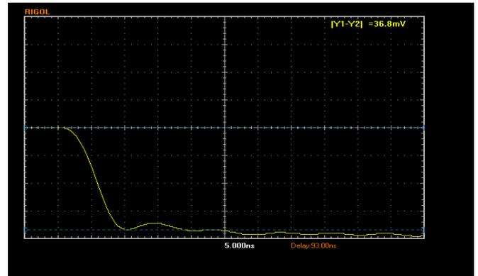
Fig. 4. Voltage of reflected waveform with short end
