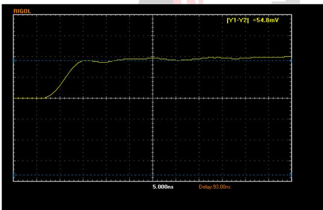
Fig. 9. Voltage of reflected waveform with 227Ω resistor
