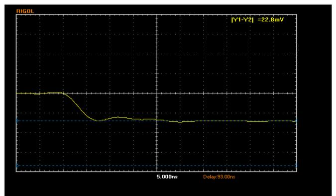
Fig. 6. Voltage of reflected waveform with 33Ω resistor
