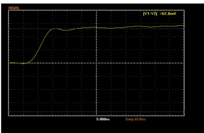
Fig. 10. Voltage of reflected waveform with 470Ω resistor
