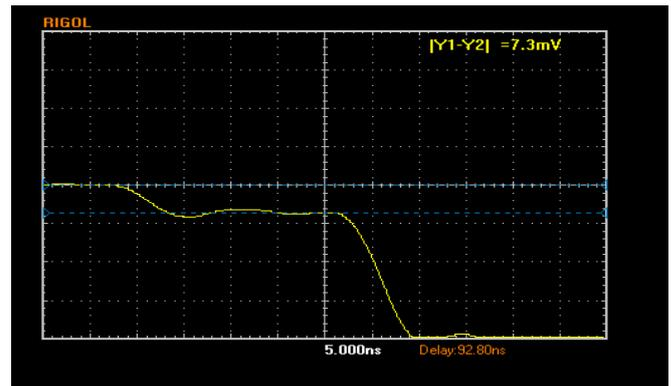
Fig. 13. Voltage of reflected waveform of 50Ω cable
