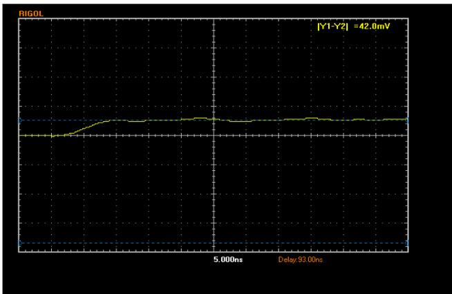
Fig. 8. Voltage of reflected waveform with 100Ω resistor
