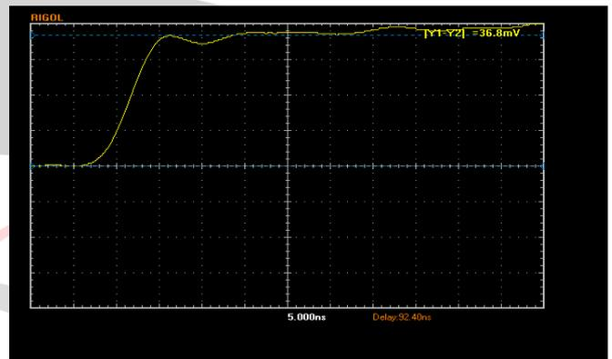
Fig. 11. Amplitude of reflected waveform with open end
