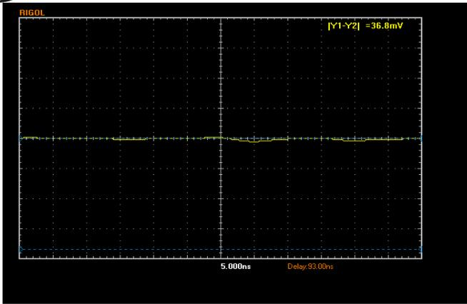
Fig. 7. Voltage of reflected waveform with 75Ω resistor
