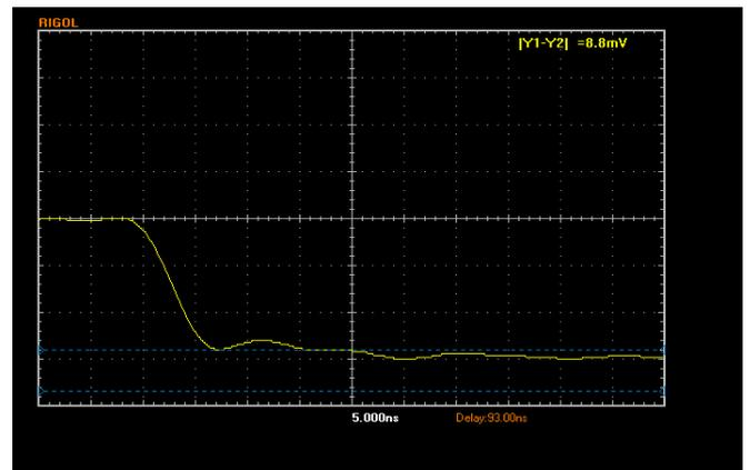
Fig. 5. Voltage of reflected waveform with 10Ω resistor
