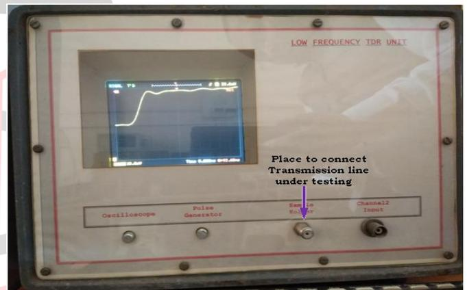
Fig. 1. Image of developed TDR
