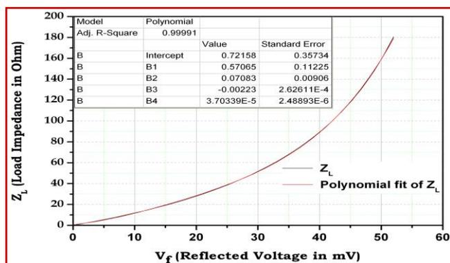
Fig. 12. Graph of  $Z_L$  vs  $V_f$
