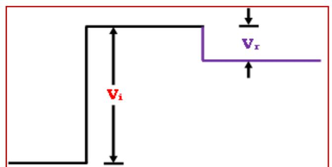
Fig. 2. Incident and Reflected waveform on TDR
