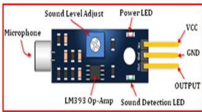
Fig. 3. Components of FC-04 sound sensor
